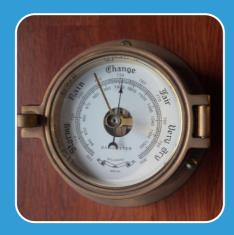
A barometer measures atmospheric pressure
