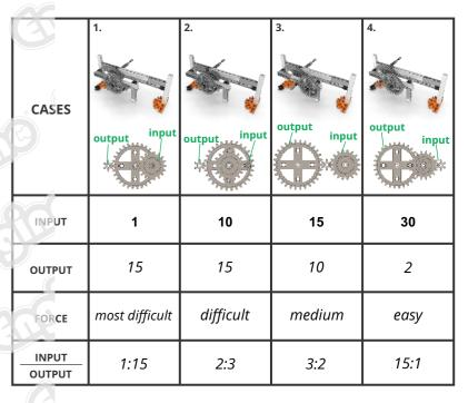
2. Why the gear ratio (input revolutions to output revolutions) is different in each case? What about Torque?
